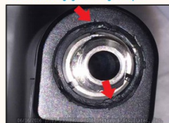
Photo 2. Scratches and gouges surrounding channel port
